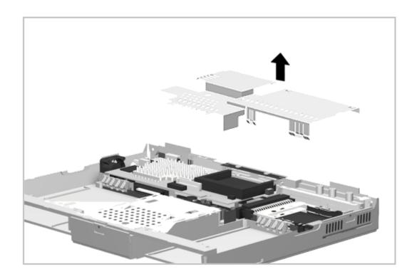
Figure 5-49. Removing the EMI Shield
